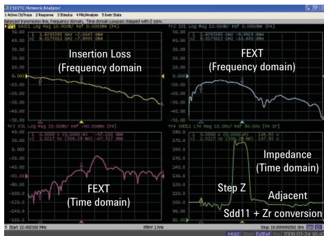
Frequency- and time-domain evaluations are shown in the same display
